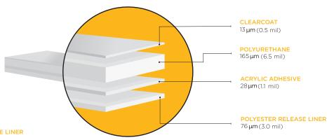
NOMINAL THICKNESS W/O RELEASE LINER 205  $\mu m$  (8.1 mil) +/- 10%
