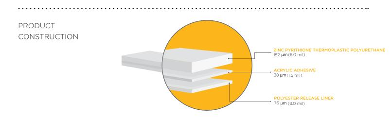
NOMINAL THICKNESS W/O RELEASE LINER 190 µm (7.5 mil) +/- 10%
