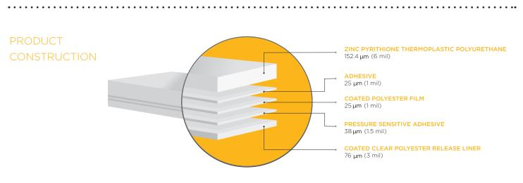
NOMINAL THICKNESS W/O RELEASE LINER 241 μm (9.5 mil) +/- 10%
