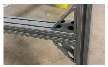
**8.** Install double to double "L" brackets to bases near center of rail, hand tightened to allow adjustment. Slide the bases brackets on to uprights, align and center, and tighten all screws.
