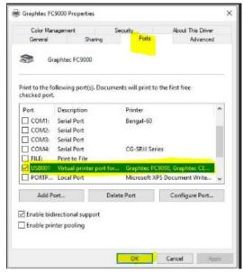
5. Unplug and reconnect the plotter, to resync the settings. Try a test cut on DAP.
